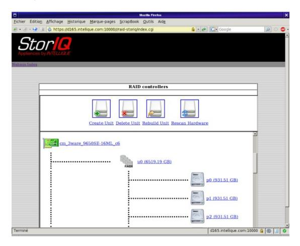
Use "Create Unit" to build a new RAID volume. The software will allow you to choose among available controllers, disks and partitions, and the possible RAID levels for the selected devices :
